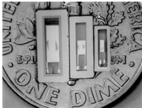
**Figure 1:** Three AT-strip resonators of three sizes. From left to right: A CX-1 a CX-3, and a CX-4.
